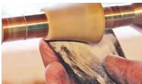
▲ The sheet abrasives are great for sanding out any lighter tool marks and can be used wet or dry
